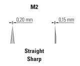
Alloy: Anti-Magnetic Anti-Acid Stainless Steel, sandblasted
