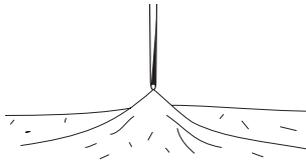
The tip consists of two very sharp, nearly horizontally opposed points. By applying gentle downward pressure and twisting slightly in a clockwise fashion, the points will embed themselves horizontally into fine membranes or skin etc., so that it may be lifted upward. This instrument also has been used successfully when separating fine tissue from an underlying area that is not to be cut.
