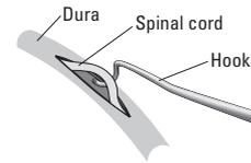
Shaped like a ligation aid and sized to isolate the spinal cord from the dura of adult mice and neonatal rats. The cord can then be cut with minimal damage to the dura.
